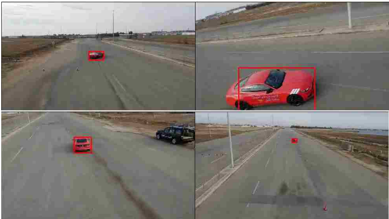
Figure 6.1: Tracking with robust detection with scale variation and high degree of appearance change
